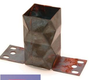
Crush-resistant. Pleated columns inspired by a beverage can are strong but lightweight -a combination that may prove useful in silos, rocket bodies, and shock absorbers.
