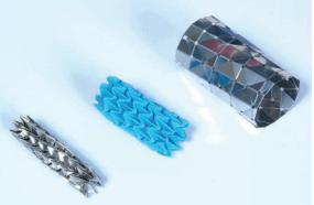
Insider. Creased stent is designed to snap open inside an artery.
