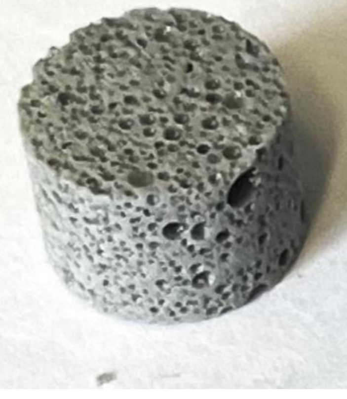
A Syntactic Foam sample used during compressive testing
