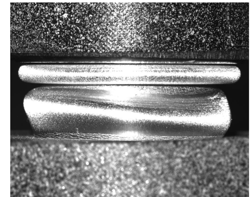
Compression of a 5mm length hollow tube; the tube deforms by forming two distinct 'Concertinas'
