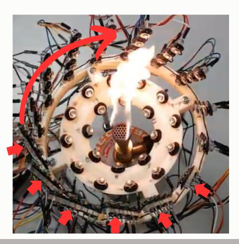
Stationary, 'pushed' flame. Active columns marked with small red arrows, rotation of active transducers marked with large red arrow.
