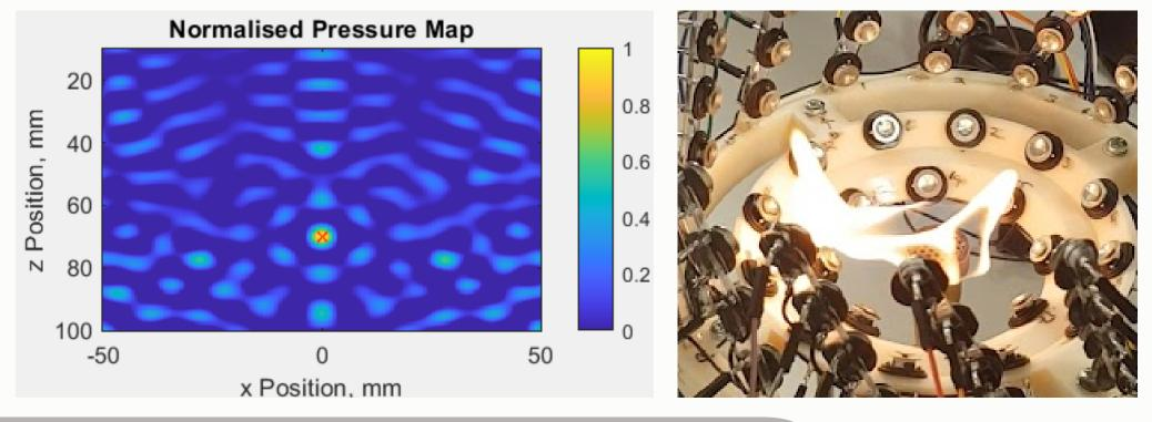
Simulated and experimental results for a single, central antinode
