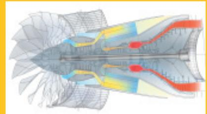
Concept design for a high overall pressure ratio intercooled turbofan engine. Rolls-Royce and the University of Oxford have researched new technologies for intercooling as part of the European Union NEWAC (New Aero Engine Core Cycles) programme. The NEWAC programme, with 40 partners from across Europe, has developed several advanced technologies that will give future aero engines reduced CO<sub>2</sub> and NO<sub>x</sub> emissions.
