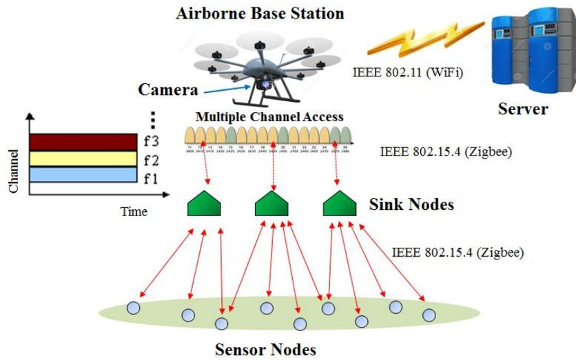
Figure 2. UAV as a local base station.
