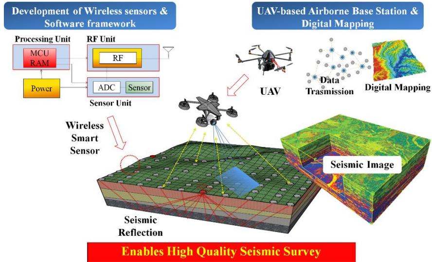
Figure 1. Proposed UAV sensor framework
