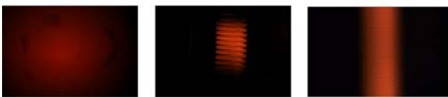
Fig. 11 Sample images from the validation experiments: black body (left), tungsten filament lamp (middle), and tungsten ribbon lamp (right)
