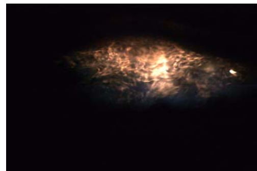
Fig. 19 Sample image from the engine in homogeneous mode, with toluene, \lambda = 0.8 , ignition timing 35^\circ before TDC, injection timing 280^\circ before TDC, image timing -10^\circ after TDC
