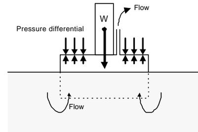
**Figure 1: Suction-assisted installation of a caisson foundation**
