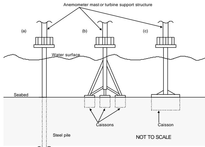
**Figure 2: Alternative designs for foundations for offshore developments**
