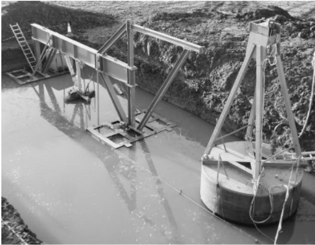
Fig. 4. Test rig, showing the 1.5 m caisson installed and 3.0 m caisson in place for installation
