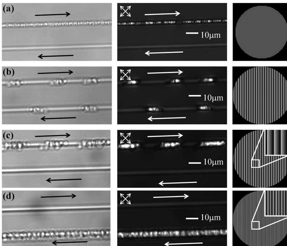
FIG. 2. Tracks written at a depth of  $170 \mu\text{m}$  in fused silica at a speed of  $10 \mu\text{m/s}$ . For each set of tracks a bright-field (left) and a crossed polarizer (centre) image are shown, as well as the phase pattern displayed on the SLM during fabrication (right). The grating period used was (a) 0, (b) 2.4, (c)  $-2.4$ , and (d) 7.2 lines per mm. Single headed arrows denote the direction of motion of the substrate for each track.
