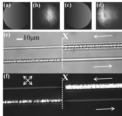
FIG. 4. Control of the pupil illumination using the SLM. (a) and (c) SLM phase distributions used to generate an intensity gradient in the pupil illumination by the zero order beam, as shown in (b) and (d). Brightfield (e) and crossed polarizer (f) images of tracks written where the SLM phase distribution is switched from (a) to (c) at point X during fabrication. Single headed arrows denote the direction of motion of the substrate for each track.
