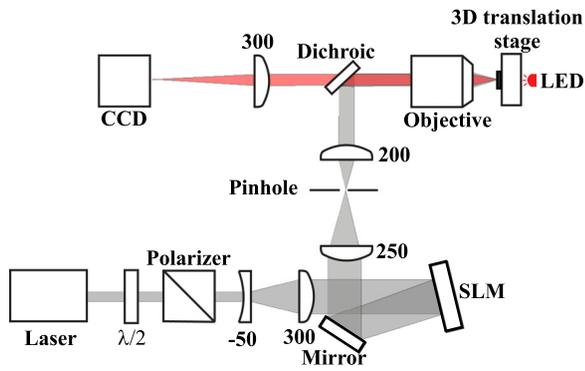
FIG. 1. The experimental configuration. All the tube lenses were achromatic doublets; focal lengths are in mm.
