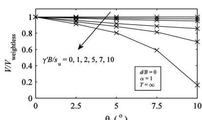
Reduction in capacity under pure vertical loading
