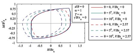
( $H, M$ ) failure envelopes for two levels of vertical loading
