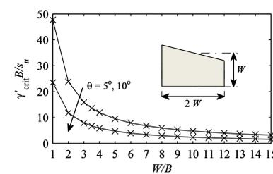
Limiting soil weight as a function of analysis domain size
