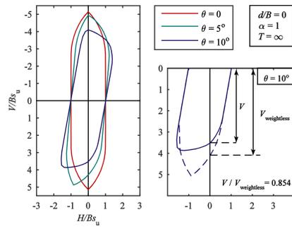
Footing on soil with weight ( $\gamma' B/s_u = 5$ )
