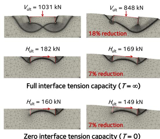
Zero interface tension capacity ( $T = 0$ )
