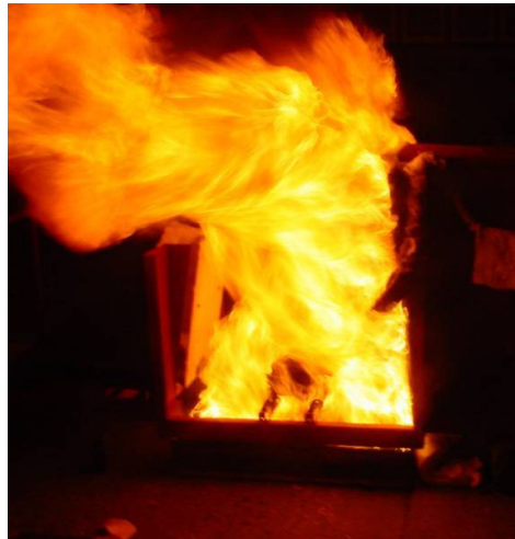
Fire test on a pultruded composite section under load
