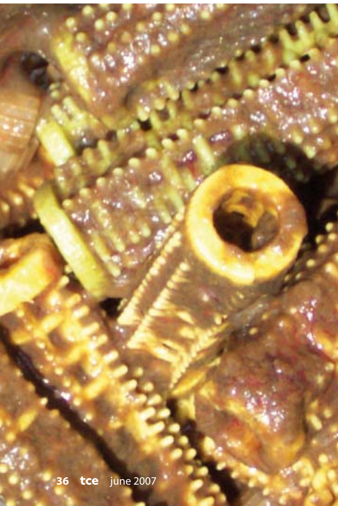
Below: Figure 5: Example of carrier media with attached biomass
